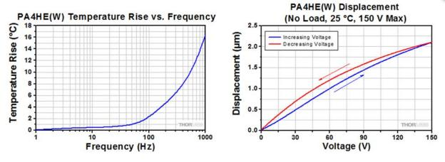
The temperature increase of the chip was measured after applying a sine-wave drive voltage, with maximum and peakto-peak amplitudes of 150 V, at the specified frequency for 10 minutes.
