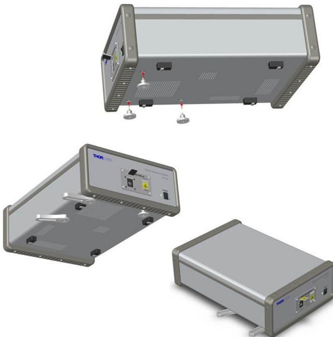
Figure 8 Attach the posts (included) and secure to the breadboard using CF175 clamping forks when using the free-space input on the OSA203B, OSA205, OSA206, or OSA207.
