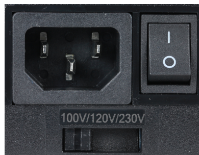
Voltage Selector Switch
