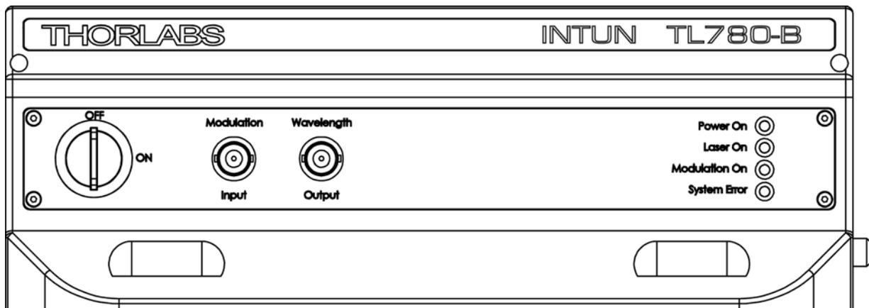
**Figure 2** INTUN Laser Front Panel
