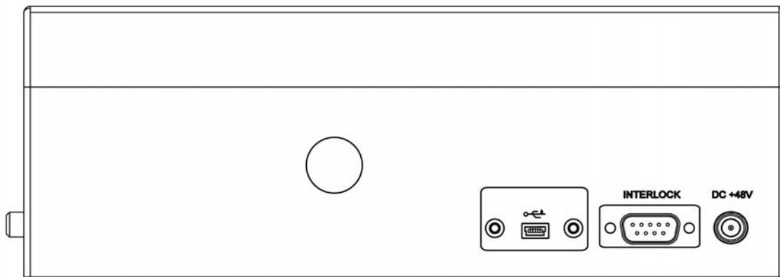
**Figure 3 INTUN Laser Rear Panel**
