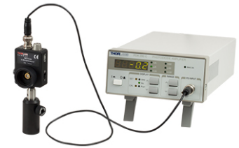
Click to Enlarge PDA200C Benchtop Photodiode Amplifier Connected to a DET10A Photodetector Using a BNC Cable
