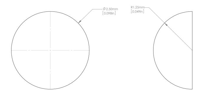
THORLABS www.thorlabs.com DRAWING PROJECTION DATE NAME 2.5MM END SPHERE JAN/14/15 YWA DRAWN MATERIAL REV A SRU JAN/14/15 APPROVAL AL2O3 COPYRIGHT © 2015 BY THORLABS APPROX WEIGHT ITEM # VALUES IN PARENTHESIS ARE CALCULATED 0.1 g **PKDESP** AND MAY CONTAIN ROUNDOFF ERRORS
