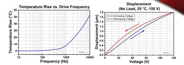
These temperature rises were measured after applying a sine-wave drive voltage ranging from 0 to 150 V at the specified frequency for 10 minutes.
