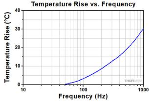
The temperature increase of the stack was measured after applying a sine-wave drive voltage, with maximum and peak-to-peak amplitudes of 150 V, at the specified frequency for 10 minutes.
