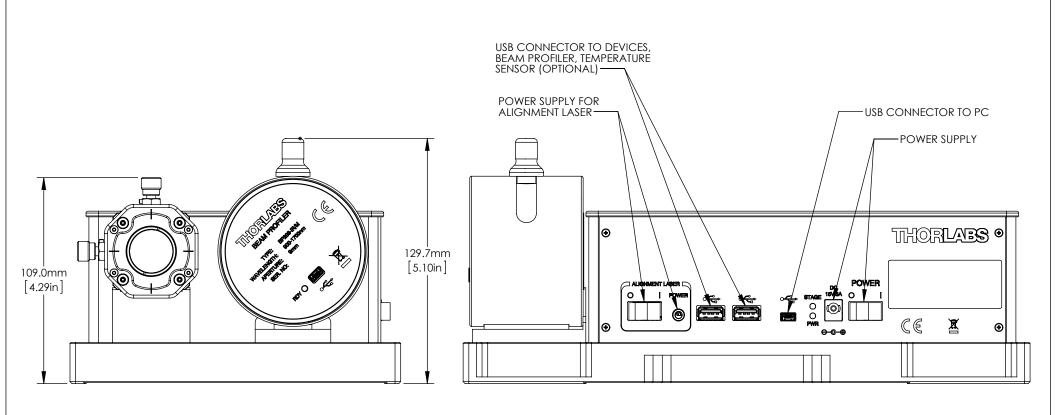
DRAWING PROJECTION THORLABS www.thorlabs.com  $\bigcirc$ NAME DATE M<sup>2</sup> MEASUREMENT SYSTEM WITH BP209-IR/M, 900-1700nm, METRIC Hit. 22/MAY/14 DRAWN RR 22/MAY/14 APPROVAL N/A COPYRIGHT © 2014 BY THORLABS APPROX WEIGHT ITEM # VALUES IN PARENTHESIS ARE CALCULATED M2MS-BP209IR/M 4.6 kg AND MAY CONTAIN ROUNDOFF ERRORS
