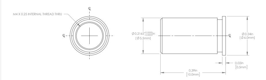
DRAWING PROJECTION  $\bigoplus$ NAME DATE M4 x 0.25 BUSHING VACUUM COMPATIBLE, 10mm LONG 20/MAR/19  $\mathsf{AK}$ DRAWN 21/MAR/19 MATERIAL REV B MJM APPROVAL PHOSPHER BRONZE COPYRIGHT © 2019 BY THORLABS APPROX WEIGHT ITEM # VALUES IN PARENTHESIS ARE CALCULATED AND MAY CONTAIN ROUNDOFF ERRORS F4MSSN2P 1.0 g
