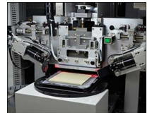
Click to Enlarge Dicing the PZT Block into Individual Elements
