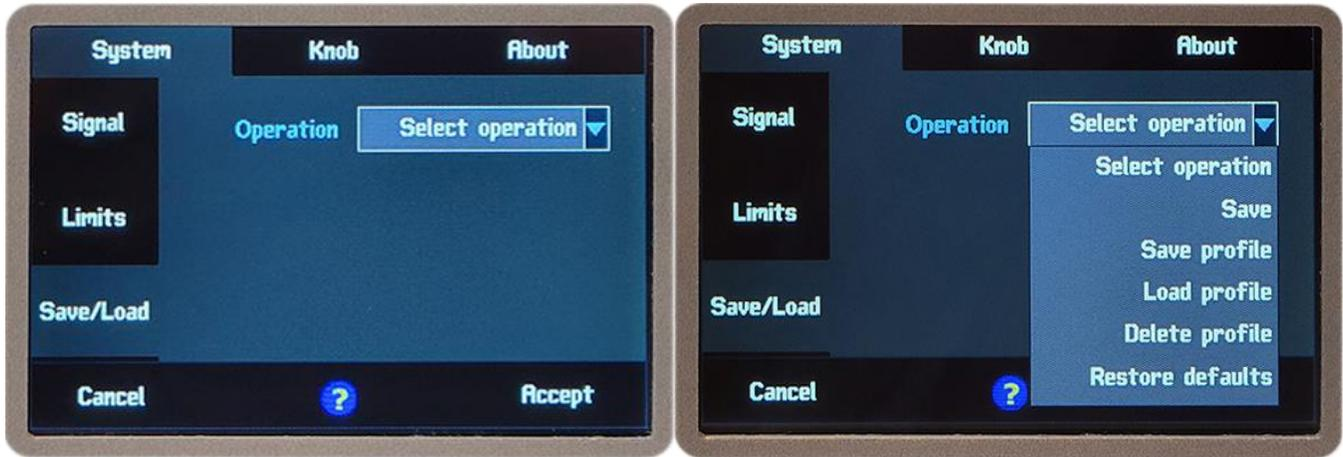
Figure 9 Save/Load Menu and Operations Dropdown Menu
