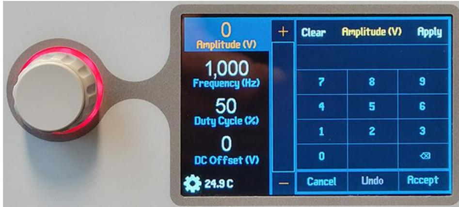
**Figure 4** Setting the Amplitude
