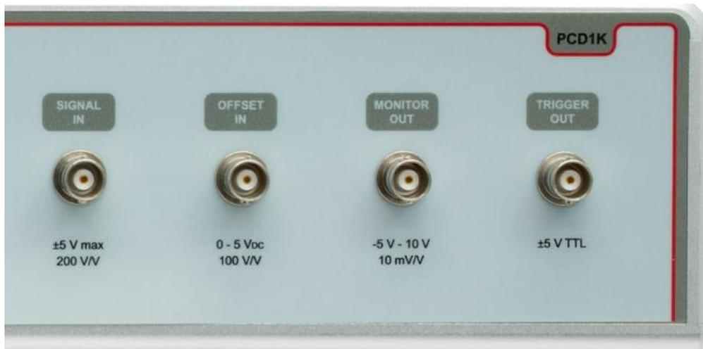
**Figure 15** Front Panel BNC Connectors
