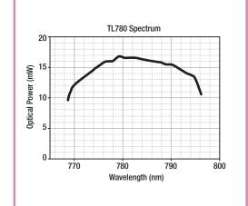
Plot of TL780 INTUN Laser Showing Optical Power as a Function of Wavelength
