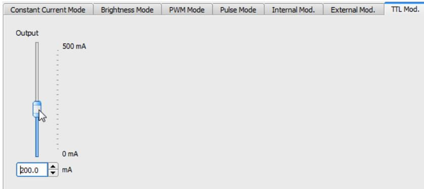
The only parameter that can be adjusted in TTL Mode is the LED current when TTL = H. The LED current can be adjusted between 0 and the LED Max. Current Limit or the User Current Limit, whichever is lower. Please see [TTL Modulation Mode](#)<sup>19</sup> for more details.
