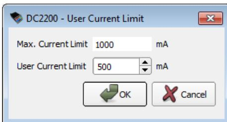
Here you can set a user current limit in the range between 1 and the displayed **Max. Current Limit** value that is read out from the memory of the connected LED (Not available for a custom LED!)
