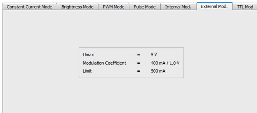
In External Modulation Mode, only the DC2200 set parameters are displayed, similar to the display shown in [External Modulation Mode](#)<sup>19</sup>.
