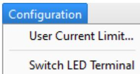
The **Configuration** menu allows the User Current Limit to be changed and the active output terminal to be switched between LED1 and LED2.
