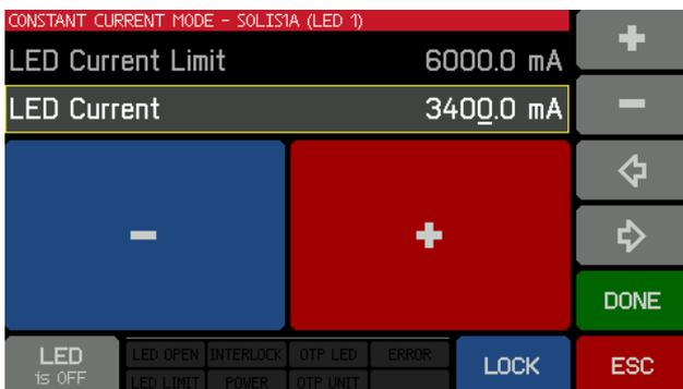
Tap the large **-** / **+** or the **-** / **+** buttons to decrease / increase the LED current. Switch LED on in order to observe the illumination.
