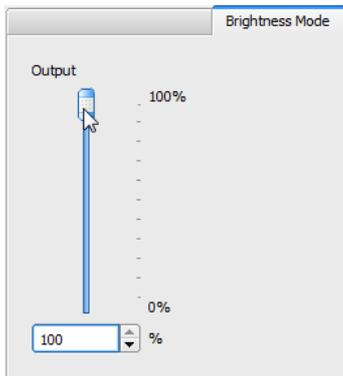
The LED brightness can be adjusted between 0 and 100%, whereas 100% refer to the LED Max. Current Limit or the User Current Limit, whichever is lower.
