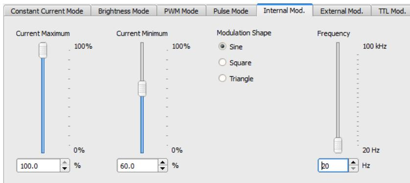
Here, the LED maximum and minimum current, the modulation waveform and frequency can be set. For details about the parameters, please see section [Internal Modulation Mode](#)<sup>18</sup>.
