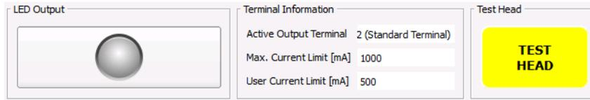
The **LED Output** button, used to switch the LED on and off, is located on the bottom of the GUI. To the right, the **Terminal Information** box displays the active terminal, the maximum current of the recognized LED and the user current limit set value. The button **Test Head** in the lower right corner proceeds a test of the LED that is connected to the active terminal, and displays the results in the [Active Terminal Information](#) dialog.
