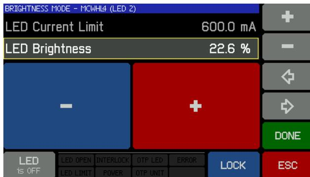
Tap the large **-** / **+** or the **-** / **+** buttons to decrease / increase the LED brightness. Switch LED on in order to observe the illumination.
