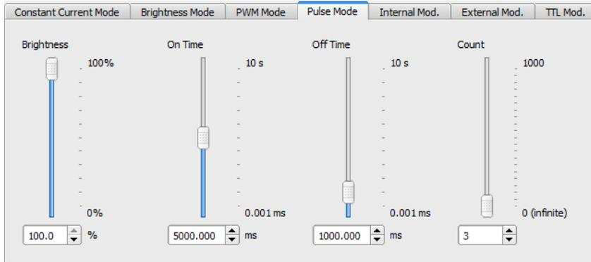
Here, the LED brightness, the LED ON- and OFF-Time and the pulse count can be set. For details about the parameters, please see section [Pulse Mode](#)<sup>17</sup>.
