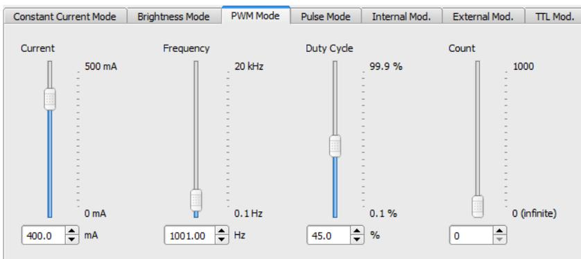
Here, the LED current, the pulse frequency, the duty cycle and the pulse count can be set. For details about the parameters, please see section [PWM Mode](#)<sup>16</sup>.
