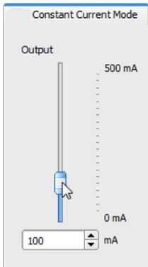
The LED current can be adjusted between 0 and the LED Max. Current Limit or the User Current Limit, whichever is lower.
