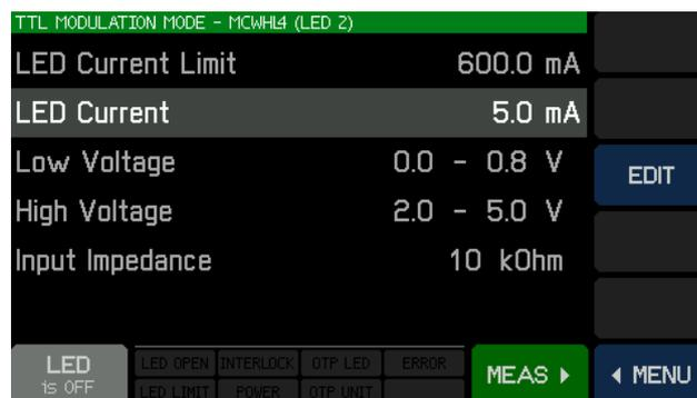
TTL Low Level corresponds to LED OFF, TTL High Level - LED ON.
