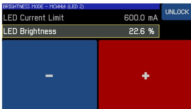
To return to normal display and make all operation buttons visible, press the **UNLOCK** button.
