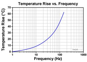
The temperature increase of the stack was measured after applying a sine-wave drive voltage, with maximum and peak-to-peak amplitudes of 100 V, at the specified frequency for 10 minutes.
