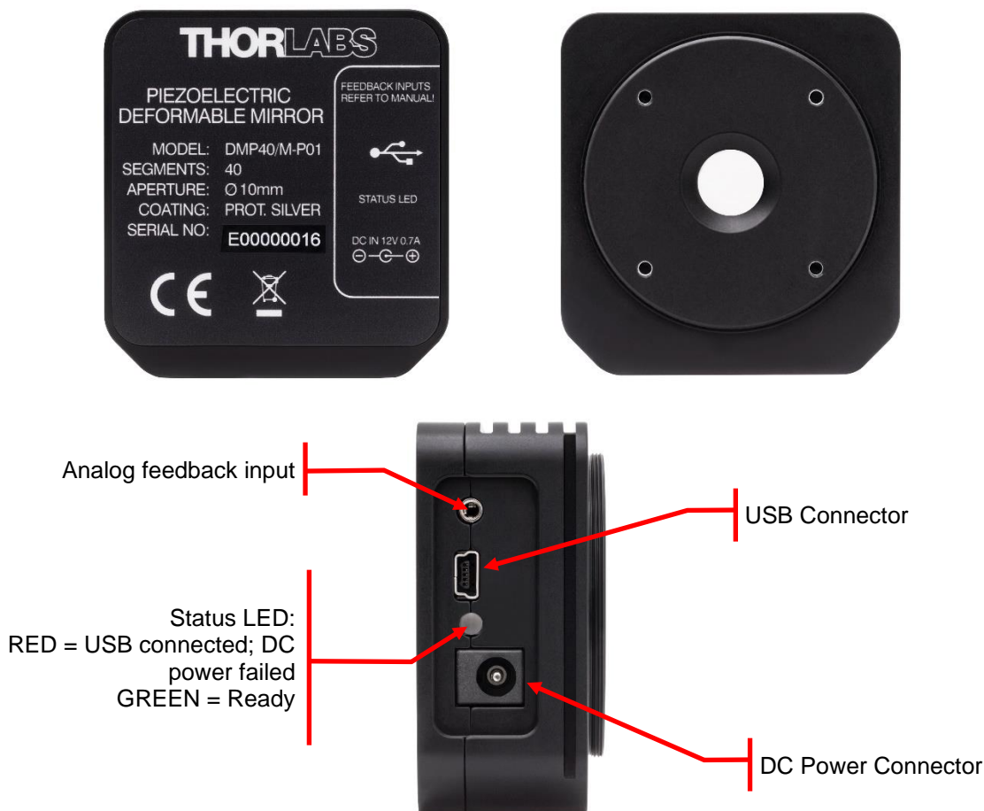
Figure 11 Piezo Electric Deformable Mirror (DMP40 shown) Connections
