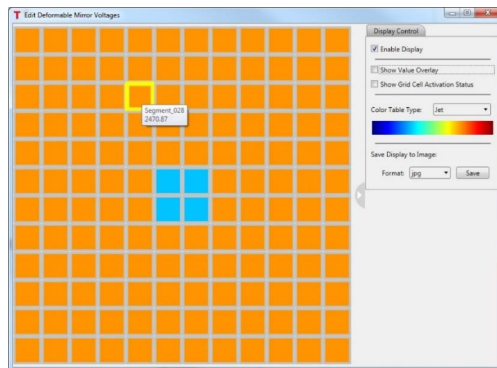
Figure 152 Hovering over a segment highlights the edges yellow and displays a box containing the segment number and displacement in microns.
