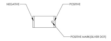
DRAWING PROJECTION THORLABS www.thorlabs.com  $\bigoplus$ DATE NAME PIEZO ACTUATOR XLIU 27/AUG/19 DRAWN 27/AUG/19 MATERIAL REV APPROVAL RG N/A Α COPYRIGHT © 2019 BY THORLABS APPROX WEIGHT ITEM # VALUES IN PARENTHESIS ARE CALCULATED AND MAY CONTAIN ROUNDOFF ERRORS PA44RK 0.6 g
