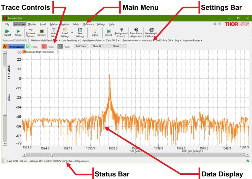
**Figure 3** The main software interface with different menu selections marked with arrows, as well as the Status bar and Data display window
