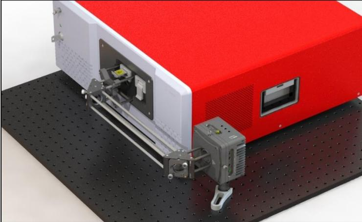
**Figure 4** Free-Space setup suitable for a Collimated Source, using a Laser Diode mounted in a Thorlabs LDM56 Laser Diode Mount. Two mirrors are used to facilitate the Alignment Process and to adjust beam height.
