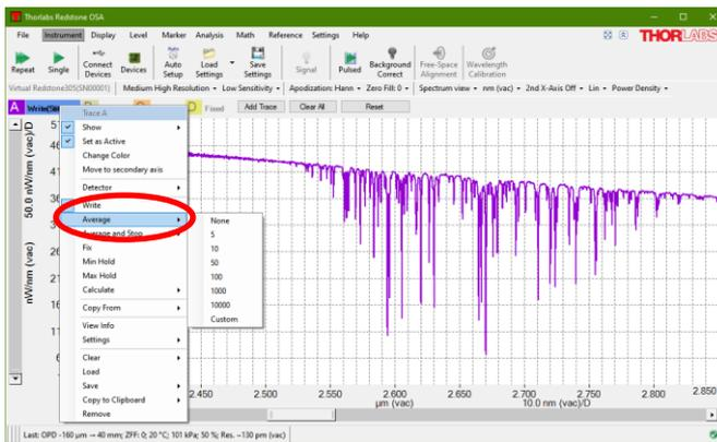
**Figure 6** The Trace Drop Down menu, with the Average option marked
