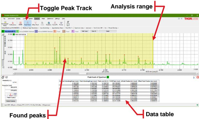
Figure 9 Peak Track Tool, used on water absorption seen in a broadband spectrum
