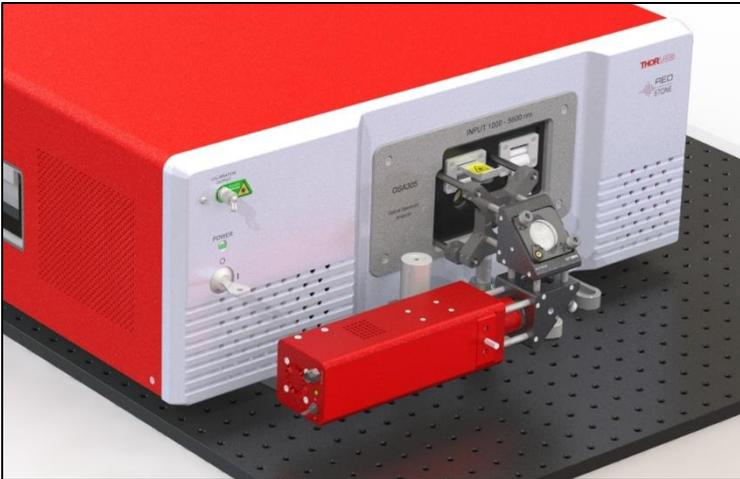
**Figure 5** Free-Space setup suitable for a Broadband Divergent Source, in this case illustrated with Thorlabs SLS203L Stabilized Light Source. The source is kept at a short distance from the OSA to minimize input losses.
