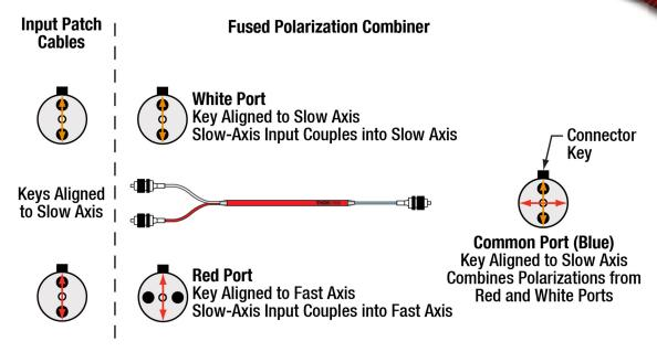
Proper alignment for splitting applications:
