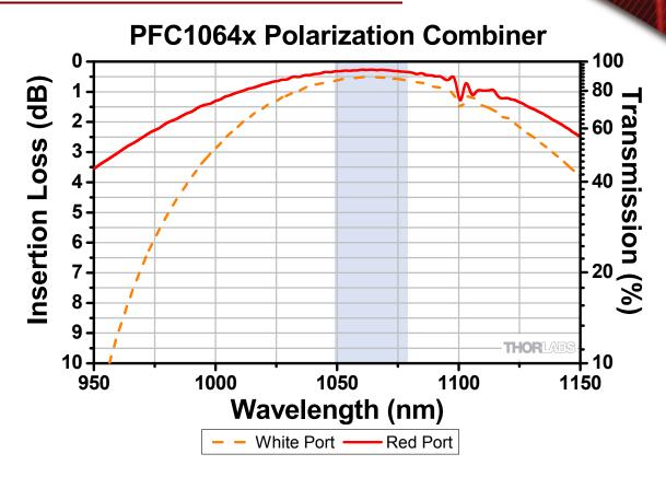
This plot shows the spectral performance of a typical 1064 nm fused fiber polarization combiner. The blue-shaded region denotes the full operating wavelength range. All data was measured without connectors.
