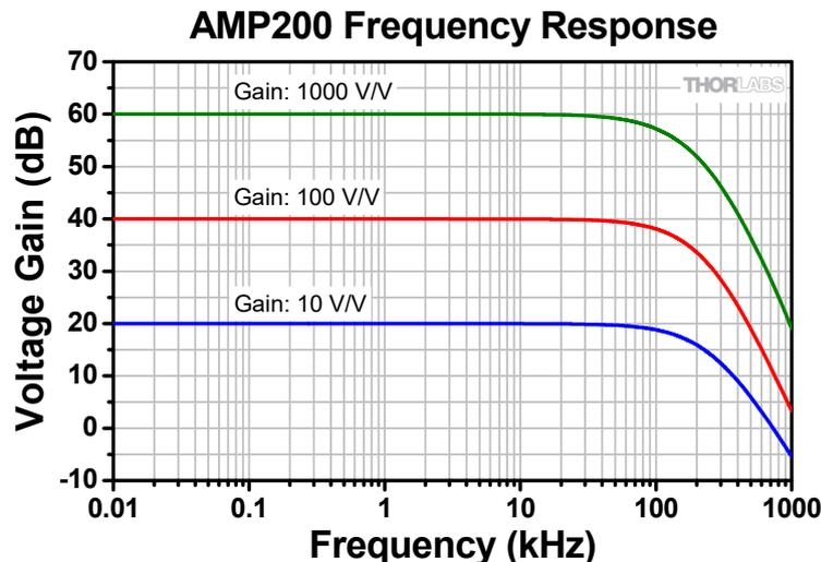
This graph shows calculated data using an input source with 50  $\Omega$  and 100 pF.
