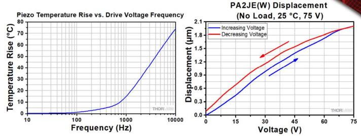
These temperature rises were measured after applying a sine-wave drive voltage ranging from 0 to 75 V at the specified frequency for 10 minutes.
