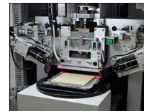
Click to Enlarge Dicing the PZT Block into Individual Elements
