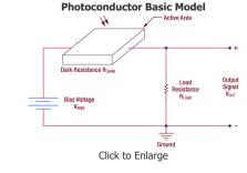
$$V_{OUT} = \frac{R_{LOAD}}{R_{DARK} + R_{LOAD}} * V_{BIAS}$$
