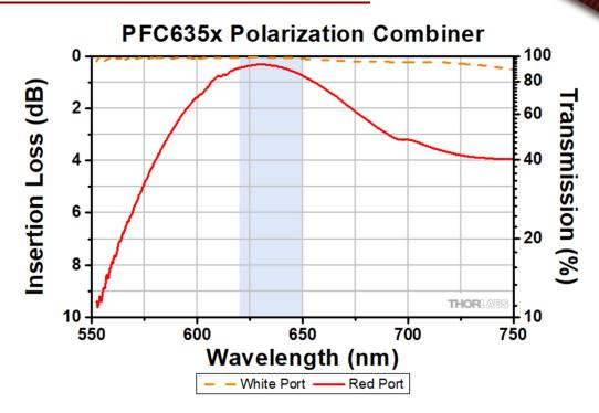
This plot shows the spectral performance of a typical 635 nm fused fiber polarization combiner. The blue-shaded region denotes the full operating wavelength range. All data was measured without connectors.
