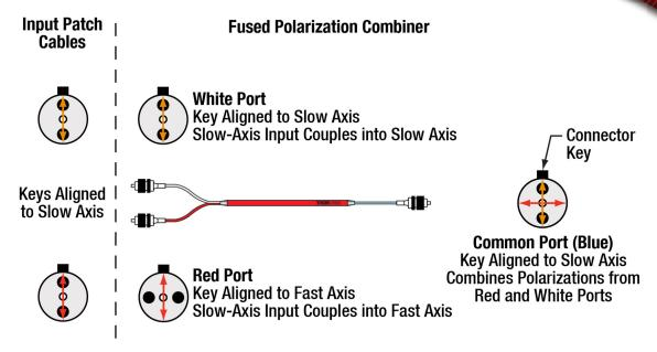
Proper alignment for splitting applications:
