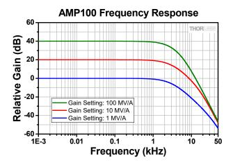
This graph represents calculated data using an input source with capacitance up to 10 nF.
