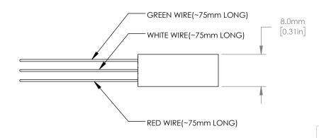
DRAWING PROJECTION www.thorlabs.com DATE NAME PIEZO ACTUATOR 24/JUN/19 ZMAO DRAWN MATERIAL REV SS 24/JUN/19 **APPROVAL** N/A COPYRIGHT © 2019 BY THORLABS APPROX WEIGHT ITEM # VALUES IN PARENTHESIS ARE CALCULATED AND MAY CONTAIN ROUNDOFF ERRORS PB4VB2W 1.3g
