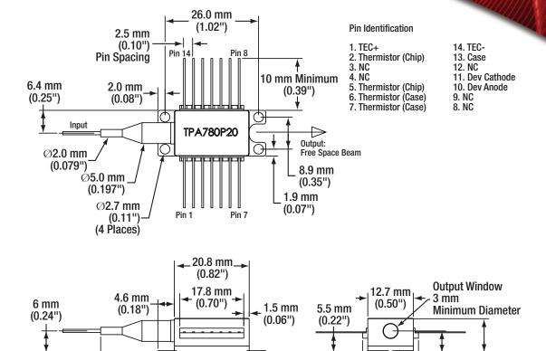
1. Device is provided with a 1000 mm length fiber tail terminated in an FC/APC connector; the fiber is Thorlabs PM780-HP fiber protected by 900 um diameter loose tube.
