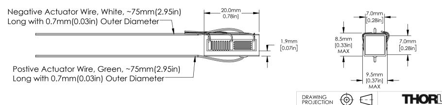
NAME DATE PIEZO ACTUATOR ΥN 26/FEB/21 DRAWN MATERIAL RG 26/FEB/21 REV APPROVAL N/A FOR INFORMATION ONLY **COPYRIGHT © 2021 BY THORLABS** APPROX WEIGHT NOT FOR MANUFACTURING PURPOSES VALUES IN PARENTHESIS ARE CALCULATED PC4GRC2 9.25g AND MAY CONTAIN ROUNDOFF ERRORS
