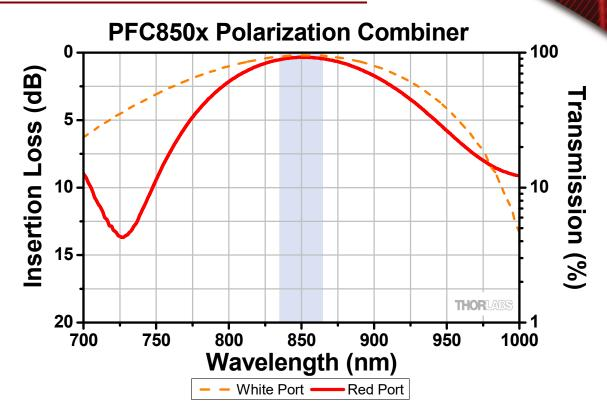
This plot shows the spectral performance of a typical 850 nm fused fiber polarization combiner. The blue-shaded region denotes the full operating wavelength range. All data were measured without connectors.
