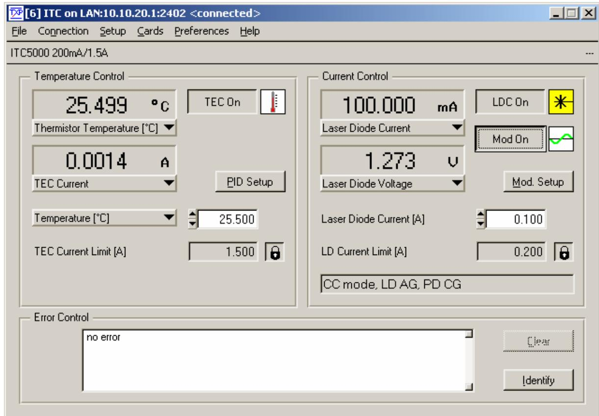
Figure 7 The ITC5000 GUI Surface
