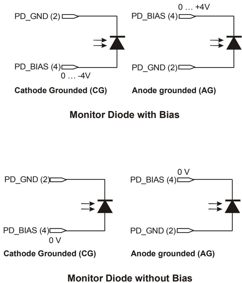
Figure 3 Connecting the Monitor Diode
