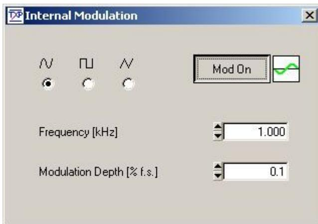
Three waveforms for the internal modulation are selectable: sine wave, square wave or triangular modulation.
