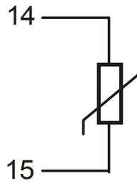
**Figure 4** Connecting the thermistor
