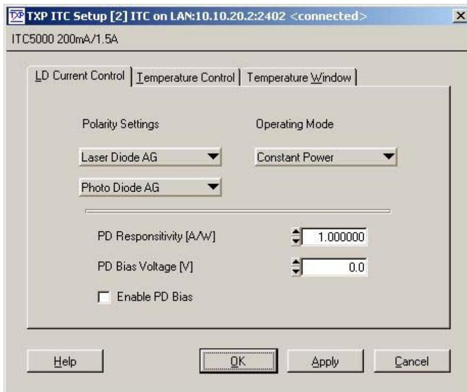
Select the correct polarity of your Laser- and Photodiode by selecting the corresponding field:
