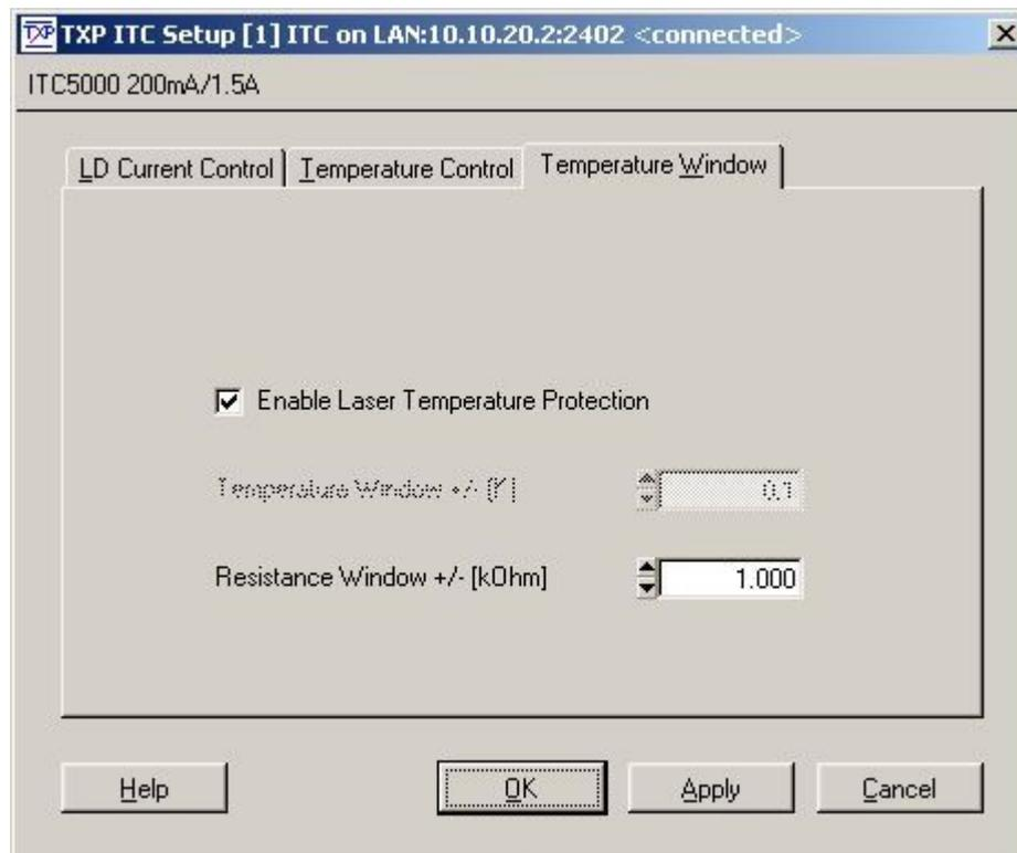
The ITC5000 allows you to set a temperature protection window. This function switches off your laser diode current, if the temperature leaves this predefined window.
