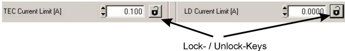
Unlock the two fields for TEC Current limit and Laser Diode Current limit, and enter the maximum allowable values for both (please refer to the data sheet of your laser diode / laser diode mount). Do not forget to lock these fields again.
