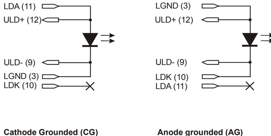
**Figure 2** Connecting the Laserdiode
