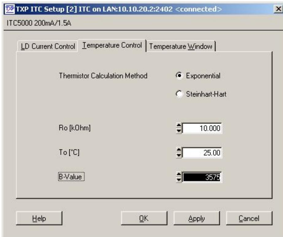
Depending on the thermistor used, the calibration coefficients are given in exponential form or as 'Steinhart-Hart'-Parameters. Select the corresponding form and enter the calibration coefficients (given in the data sheet of the thermistor / Laser Diode).
