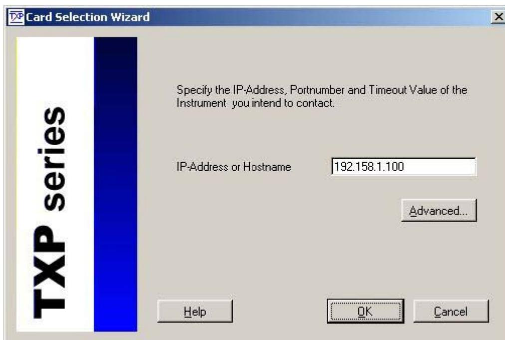
Enter the IP Address of your TXP mainframe (this address is given to the TXP in the initialization process with the TXP-Administrator program) and if necessary (ask your system operator) also the port number and a timeout value under 'Advanced':
