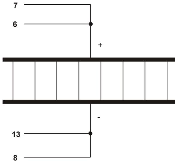
Figure 5 Connecting the TEC
