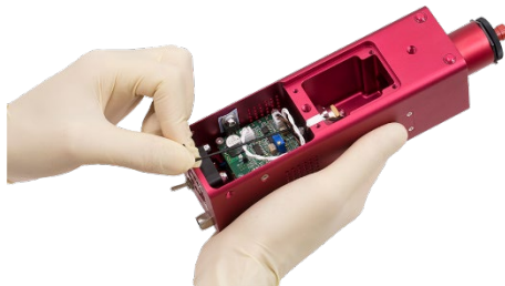
Figure 16 Loosen the bulb module locking screw.
