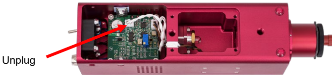
Figure 17 Unplug the bulb module connector.
