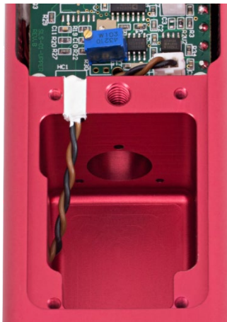
Figure 20 Holes on the Central Wall for Bulb Dowel Pins
