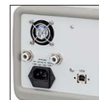
Click to Enlarge Rear-Mounted Hose Connections Around Power Connector
