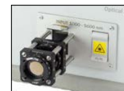
Cage-Mounted Polarizers in Front of Free-Space Input
