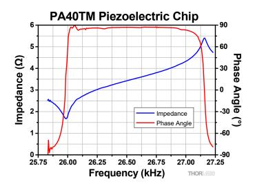
This data was acquired under no load at 25 °C by an impedance analyzer with frequency sweeping.
