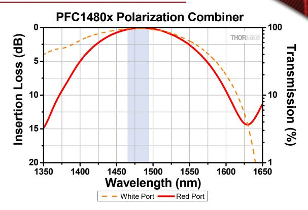
This plot shows the spectral performance of a typical 1480 nm fused fiber polarization combiner. The blue-shaded region denotes the full operating wavelength range. All data were measured without connectors.
