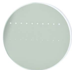
The photograph above is a protected aluminum-coated mirror after LIDT testing. In this particular test, it handled 0.43 J/cm 2 (1064 nm, 10 ns pulse, 10 Hz, Ø1.000 mm) before damage.
